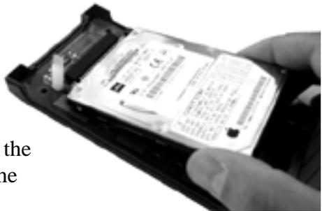
**Step 5:** Refer to the picture at the right. With your thumbs, carefully but firmly push the hard drive forward to complete the insertion of the hard drive pins into the IC board connector.
