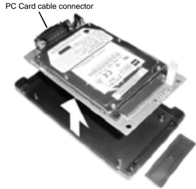
**Step 7:** Making sure that the hard drive does not fall from the IC board, flip the IC board/hard drive assembly over and screw in the 4 short metric screws which secure the drive onto the IC board.
