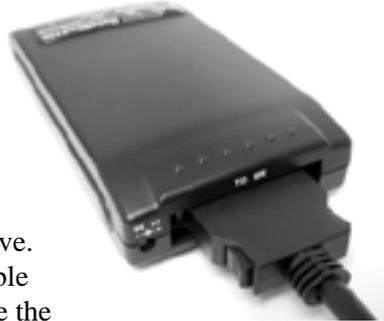
The DataShuttle Xtreme drive will begin to spin once it receives power through the PC Card slot. If your computer is powered on, the drive will activate and mount onto your computer's Desktop automatically. You can now use the DataShuttle Xtreme drive as you use any other Mac OS hard drive.
