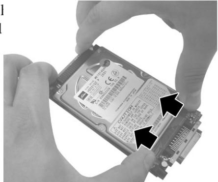
**Step 7:** Making sure that the hard drive does not fall from the IC board, flip the IC board/hard drive assembly over and screw in the 4 short metric screws which secure the drive onto the IC board.
