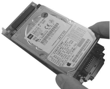
**Step 6:** Referring to the picture 1 carefully but firmly push the hard drive forward with your thumbs to completely insert the hard drive pins into the IC board connector.
