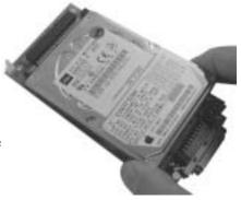
**Step 6:** Referring to the picture here, carefully but firmly push the hard drive forward with your thumbs to completely insert the hard drive pins into the IC board connector.
