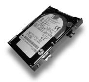
**Step 6:** Carefully attach the Drive Connector to the hard drive as shown here. Looking from above the hard drive, note that the two left-most columns of pins (four pins total) are <u>not</u> connected to the Drive Connector. Do not place a jumper on the unconnected pins.
