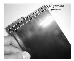
**Step 12:** Before securing the final screws, ensure the Drive Connector is properly aligned and is not crooked or loose in its slot.
