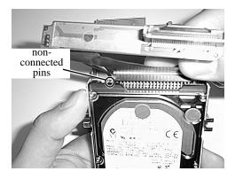
Step 7: Gently lay the hard drive with bracket onto the four rubberized mounting posts in the Kit Base.
