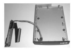
**Step 3:** Carefully lift the Silver Internal Hard Drive Bracket and the bag of screws from out of the Kit Bottom, being careful not to snag the LED wires. Remember the orientation of the Drive Bracket relative to Kit Base.
