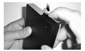
**Step 13:** Once the Kit Top and Drive Connector are properly aligned with the Kit Base, secure the Kit Top to the Kit Base by screwing the five top-mounted flat head screws into position.
