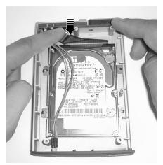
**Step 11:** Next, place the black Kit Top onto the Kit Base. Notice the alignment groove located on the inside rear of the Kit Top.
