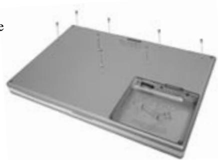
**Step 5:** Remove the base plate by sliding it towards the front of the computer about a half inch, releasing its inner latches, and then up and away from the main chassis.
