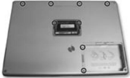
**Step 9:** Remove the three screws on each side of the computer starting with the screws closest to the back of the computer and working your way forward. **Note:** Be sure to replace these screws in this same order when closing the computer.
