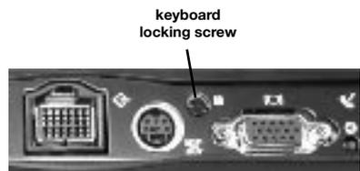
**Step 6:** Push the keyboard front of the PowerBook and gently lift so that the keyboard pops up from that end. Disengage the tabs on the bottom of the keyboard which secure it to the palm rest by holding the top corners of the keyboard and pulling them up and out.
