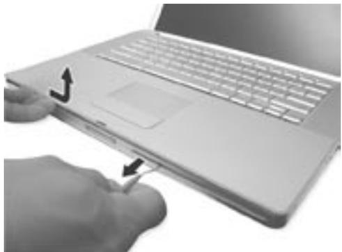
**Step 14:** Lift the front of the top case and gently lay it against the the display, careful not to strain the cables connected to the logic board underneath the top case.
