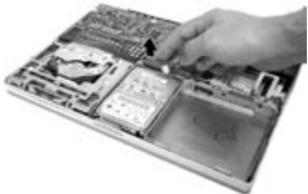
**Step 8:** Remove the hard drive from its bay by first lifting the side of the hard drive from which the two screws were removed up and out, and then lifting the rest of the drive out of the bay.
