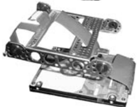
**Step 16:** Carefully remove the ribbon cable connector from the hard drive.
