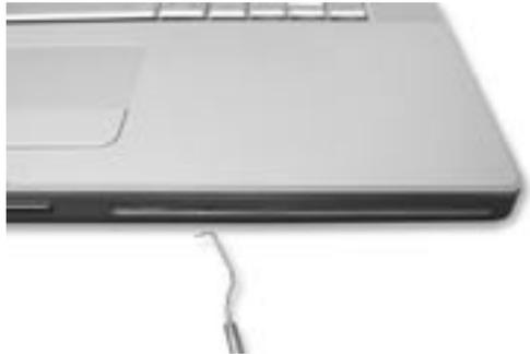
**Step 13:** Insert the pick tool into the optical drive slot behind the clip and carefully pull out to release the clip and the top case. You may need to carefully but firmly lift the front edge of the top cover to release it from the bottom case.
