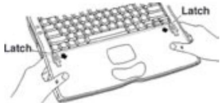
**Step 6:** Slide the keyboard about a half inch toward the front of the computer until the five metal tabs on the back of the keyboard clear the chassis.
