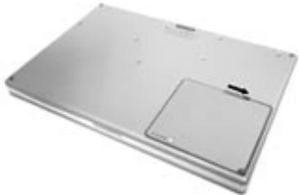
**Step 4:** Using the Phillips end of the MCE mini screwdriver, remove the eight screws from the base of the computer.
