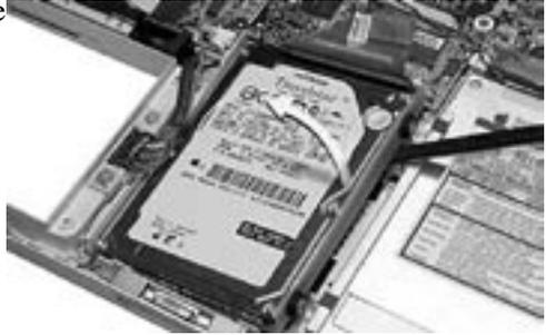
**Step 23:** Remove the logic board cable, plastic shield, rubber grommets, and side screws from the original internal hard drive and place them onto the new hard drive.
