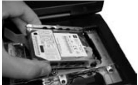
**Step 12:** Remove the four screws from out of the black grommets at the side corners of the hard drive bracket using the Torx T8 driver.
