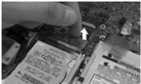
**Step 21:** Carefully disconnect the hard drive cable from the logic board by prying its connector upward using a fingernail.
