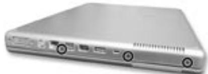
**Step 10:** Remove the two top screws on the back of the computer.
