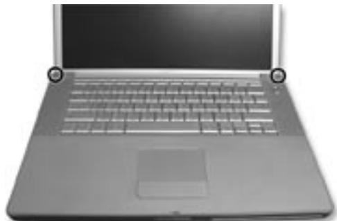
**Step 12:** Pry the top part of the case from the bottom by running your fingernails or some other non-marking wedge along the seam that goes around the case, starting from the back and moving forward.
