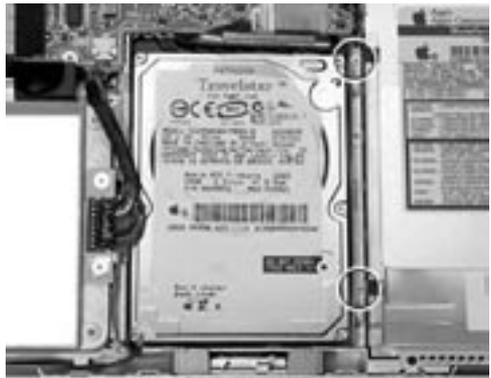
**Step 19:** Lift the bracket out of its slot.
