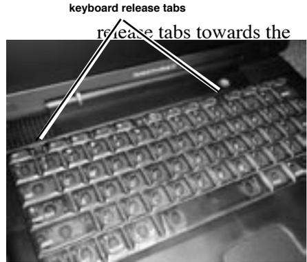
**Step 7:** Carefully rotate the keyboard so that it lays face down on the PowerBook's palm rest, being careful not to pull on the ribbon cable attaching the keyboard to the logic board.
